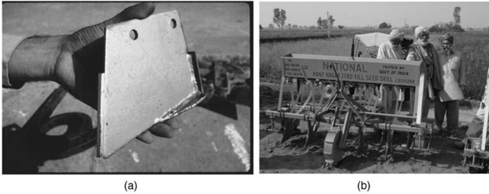
Figures 3. (a) and (b): The NZ inverted-T opener and the locally manufactured Indian seed drill with these openers (Photograph: Peter Hobbs).
